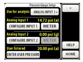
At this point the pressure transducer is reporting the transducer pressure to the BGA244. Press [Home] and verify that the pressure reading is in psi(a). If the transducer is open to air it should read the local atmospheric pressure (14.7 psi(a) at sea level).
